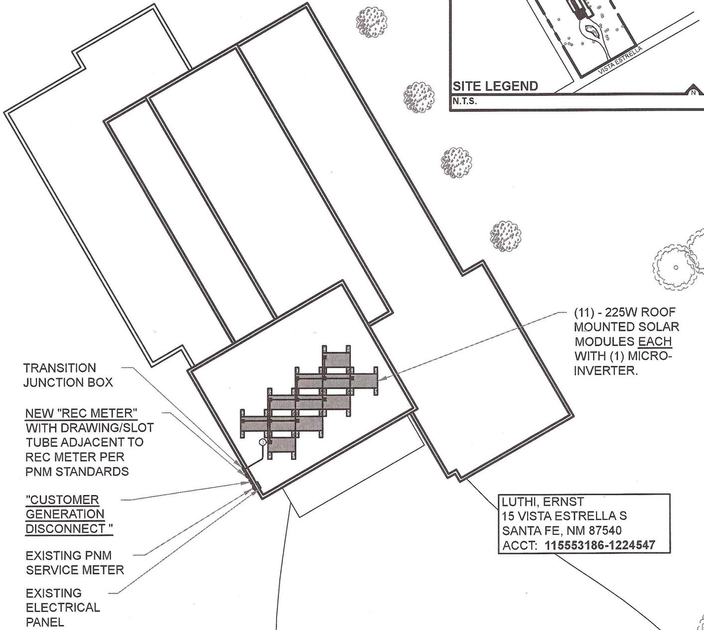
(11) - 225W ROOF MOUNTED SOLAR MODULES EACH WITH (1) MICRO-INVERTER.
