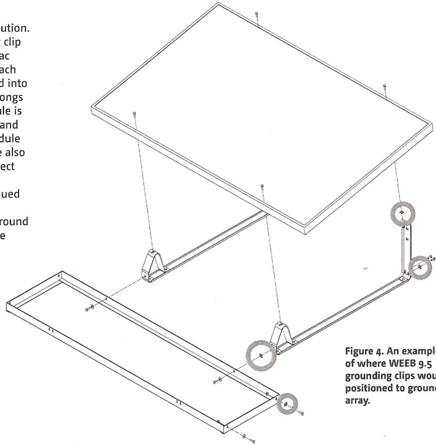
Figure 4. An example of where WEEB 9.5 grounding clips would be positioned to ground an array.
