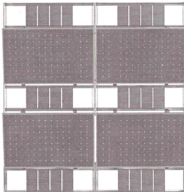
**Note:** Unirac requires that all perimeter ballast blocks be adhered to the bay with Subfloor construction adhesive (BC-490 or equal).
